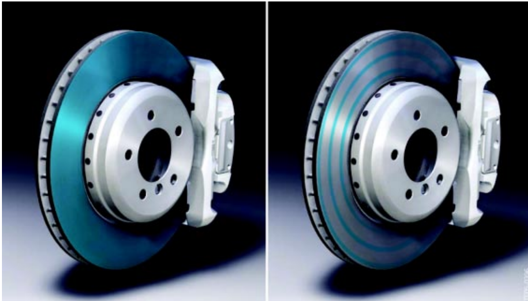
Left Brake Disc with Water Film before Dry Braking Right Brake Disc After Dry Braking
